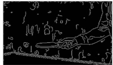
(c) 二级双边滤波后边缘 (c) Extracted edge after two-scale bilateral filtering
